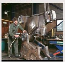
Demolition tools is a typical application where HARDOX HiTuf exellent performance is utilised.
