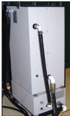
Oil Heater/Chiller Unit
