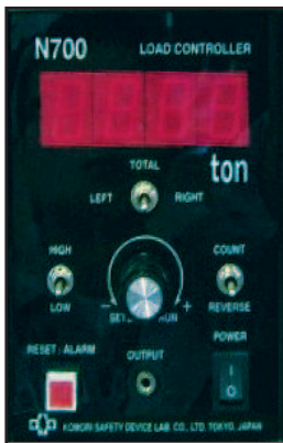
Load Monitor Screen
