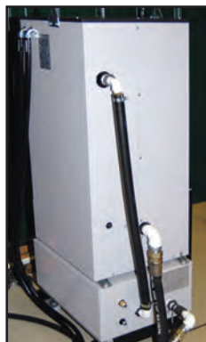
Oil Heater/Chiller Unit
