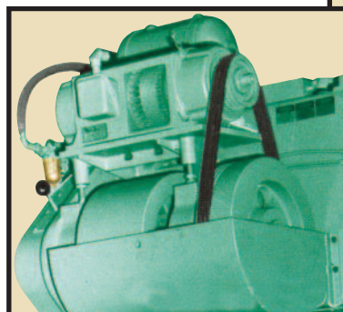
Geared Drive Motor is on rear as shown.
