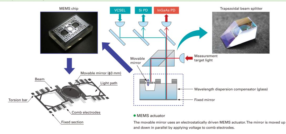
Ultra-compact near infrared spectrum sensors that integrate MEMS-FPI tunable filter and photosensor
