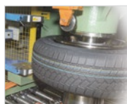
Retrofit Tire Uniformity Line RTU
