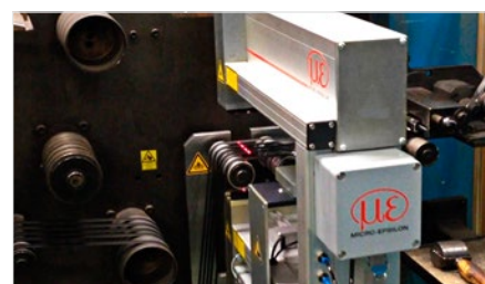
C-frame profilometer in production environment
