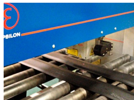
Thickness measurement with TCP 8301.CT
