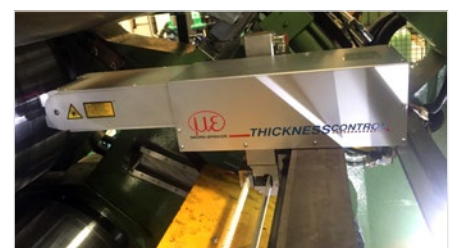
Sensor in measuring position in calender
