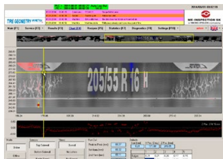
Visualization of sidewall inspection
