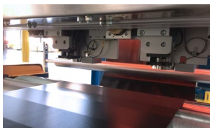
thicknessCONTROL TCP 7303.ET view in product direction
