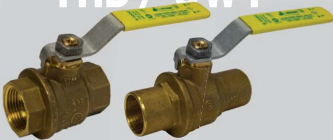
T/S-100C: Two-Piece Lead Free Brass Ball Valve - Full Port, 600 WOG Available in sizes 1/2" - 2"
