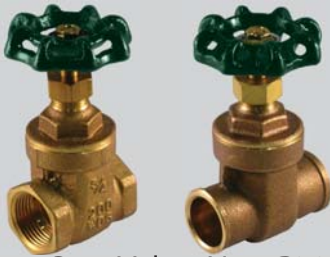
T/S-301G: Brass Gate Valve, Non-Rising Stem, 200 WOG Available in sizes 1/4" - 4"
