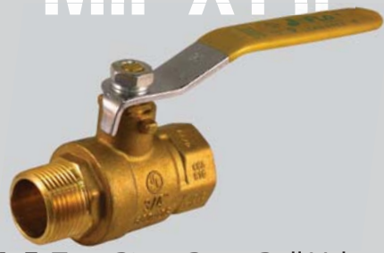
JF-100GMxF: Two-Piece Brass Ball Valve - Full Port, 600 WOG Available in sizes 1/4" - 1"
