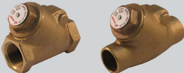
T/S-511G: Bronze Y-Pattern Check Valve - 300 PSI Available in sizes 1/2" - 3"
