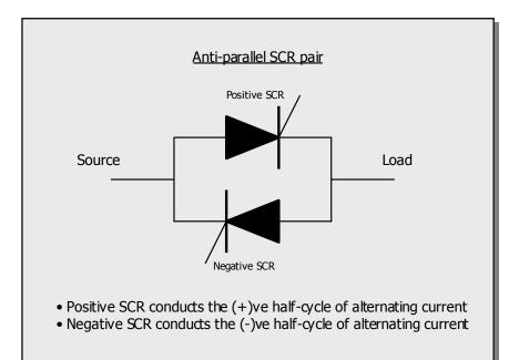
Figure 3: Anti-parallel SCR pair for AC waveform
