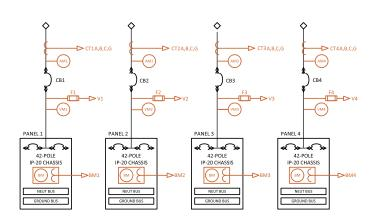
Series 70: eRPP - 4 Input 4 Panel Feed-Through Configuration
