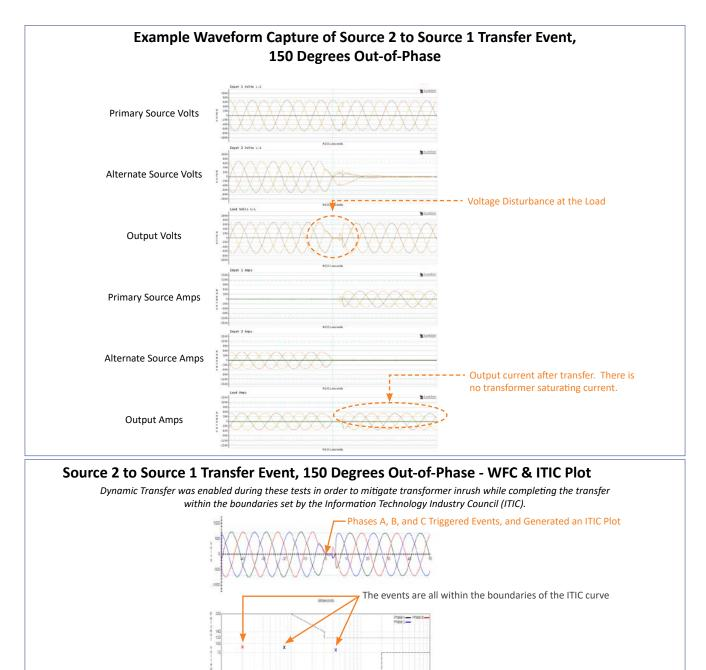
The ability to keep the transfers within the ITIC limits was verified through the Voltage Disturbance Analysis Tool (VDAT) plot shown above in the captured waveform.
