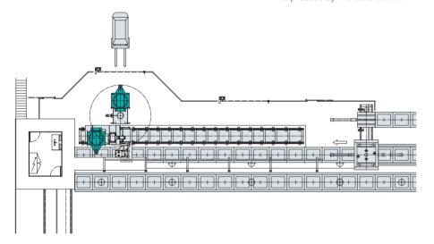
High-tech manufacturing foundry: typical layout of MX 30 pouring machine, fully automated version.
