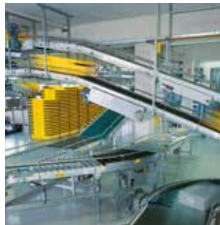
Secure inclined conveying due to conveyor belts with patterns or lateral profiles.
