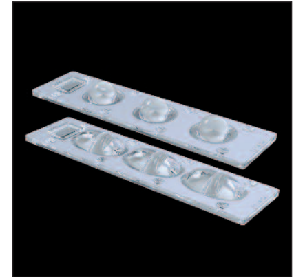
PL0333 IESNA Type I - Full angle at 50% from maximum: ~ 150°x90° - Full angle at 10% from maximum: ~ 160°x100°
