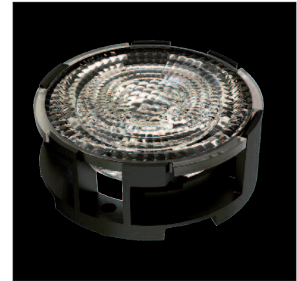
PLL2008WI 42° FWHM – Full angle at 50% from maximum: ~ 60° – Full angle at 10% from maximum: ~ 160°
