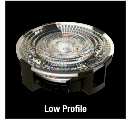
PLL2010WI 42° FWHM – Full angle at 50% from maximum: ~ 60° – Full angle at 10% from maximum: ~ 160°
