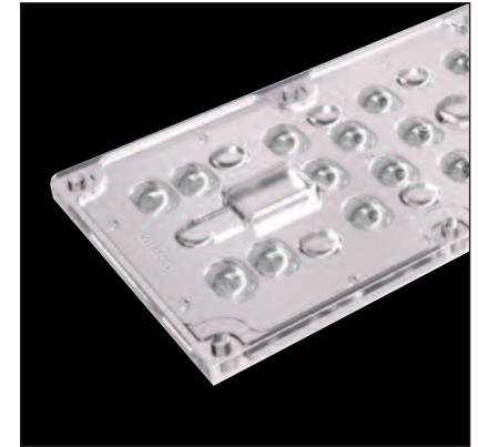
PLL240003 IESNA TYPE V - Full angle at 50% from maximum: ~ 150° x 150° - Full angle at 10% from maximum: ~ 170° x 170°
