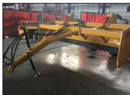
6" x 6" x 3/8" Wall Tube for Crossmember and Tongue
