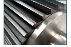
Cutting tools can be optimally adjusted to your requirements; cutting rotors of hardened chromium steel, of sintered PM steel or with clamped or soldered HM blades
