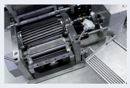
Strand infeed area – designed for ease of cleaning
