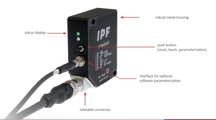
No greater flexibility exists: The connector of the **PT64** can be rotated up to 180°.
