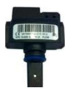
The *ITC Smart Manifold* is equipped with very compact sensors that are capable of reading both flow rate & temperature. The sensor is based on the vortex flow measurement principal, which uses a bluff body in the middle of the flow path to create a small eddy current (vortices) and the pressure of this current is measured to determine the flow through a given cross sectional area with an accuracy of  $\pm 1.5\%$
