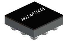
Scale to size Tiny UTQFN-9 Package 1.5x1.5 mm
