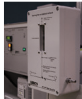
HT/HP inlet (up to 30 bar at 200°C)
