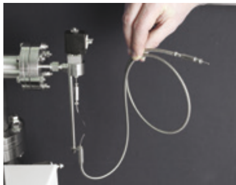
Micro-flow capillary inlet. Sampling rate 12 \mu\text{l}/\text{min} . Single or multi-capillary inlet option
