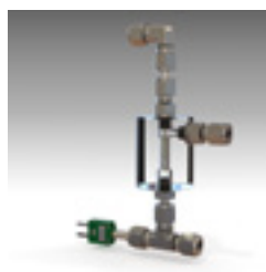
Interchangeable membrane inlet probe types
