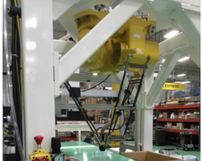
Figure 8: Robotic subsystem represents an integral part of the machine vision system and must communicate seamlessly and in real-time with the hyperspectral sensor, using industry-standard protocols.
