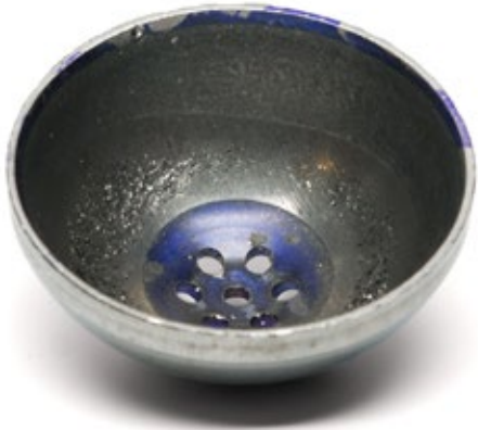
Inner Race after 3,800 lbs / 1,700 kg rolling load test. No damage to Weep Holes.
