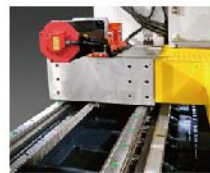
X travel by rack pinion servo control (2 pcs)
