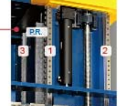
Each column with 3 linear guide-ways and 1 position rail (P.R.) (Patent NO. M511389)
