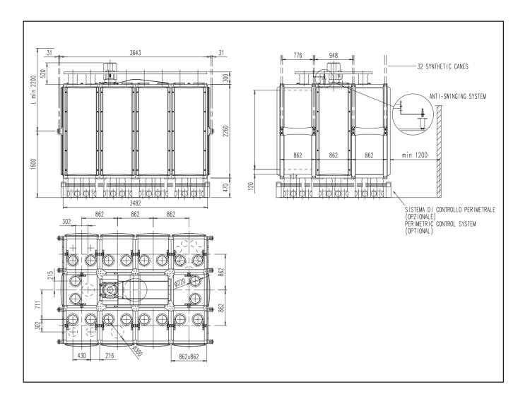
Sieve dimension = 740x740mm Net sieve surface = 0,41 mm<sup>2</sup>
