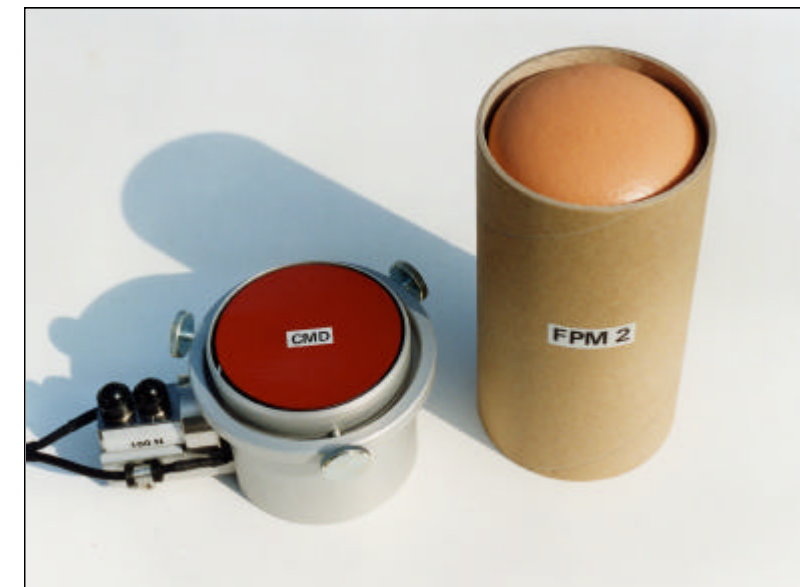
Fig. 4: The polarization sensor CMD, which is integrated into the FPM device measures the dielectric polarization of a foam sample simultaneously with the rise pressure. patent 10104854
