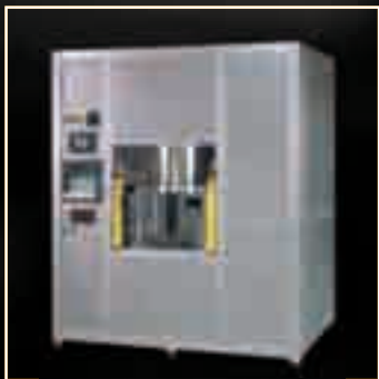
Vacuum Furnace for controlled atmosphere brazing
