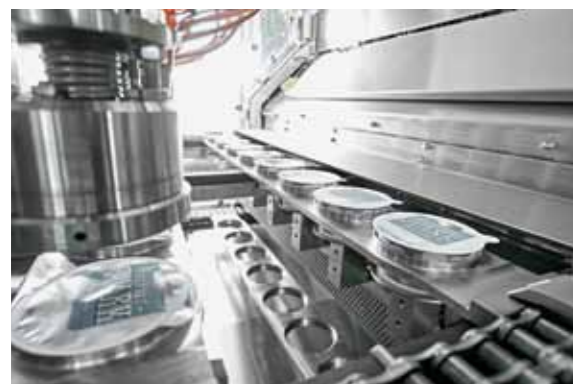
(3) Photo on the left: sealing station
