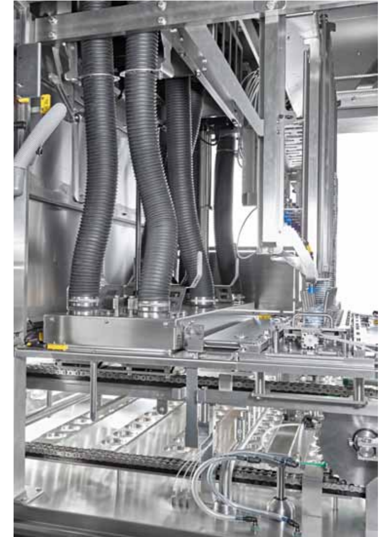
Photo above: Double pulsed light high-performance UV(C) cup sterilisation with guaranteed sterilisation rate LOG 4
