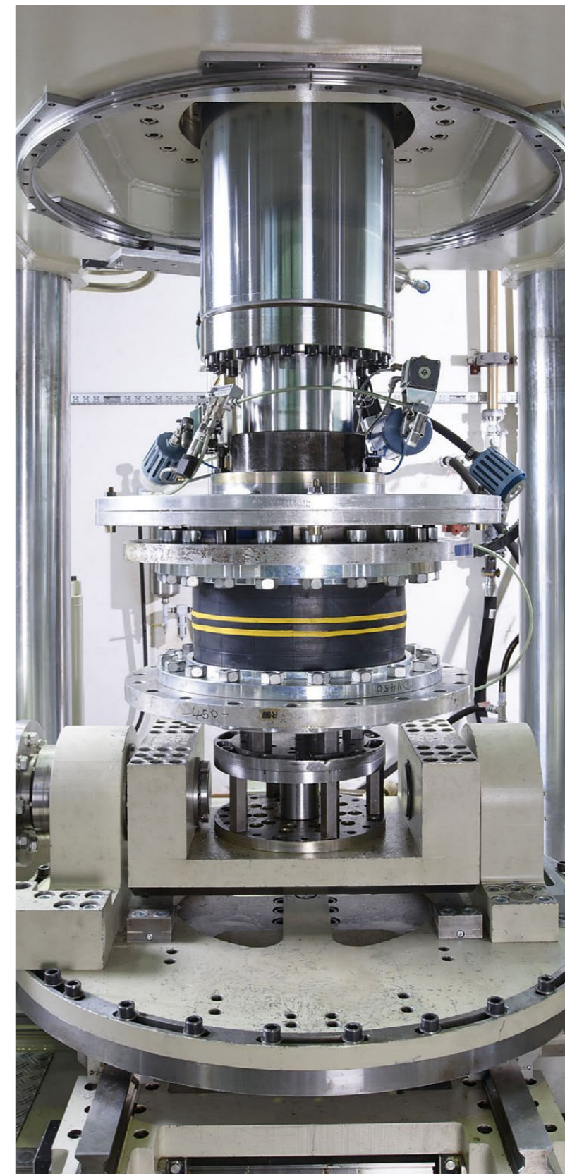
Multifunctional test rig – photo showing extreme elongation
