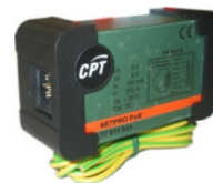
Fig. 13. PoE protector for CCTV, with power supply and communications in a single conductor.
