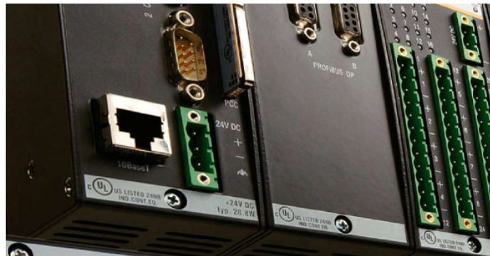
Fig. 5. PLC input, output and communication lines, highly sensitive to surges
