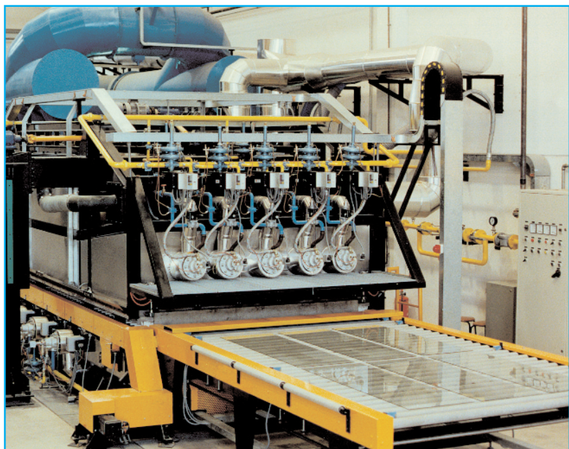
Glass tempering furnace with recuperative, radiant burners, model SER (Poppi Eurotech)
