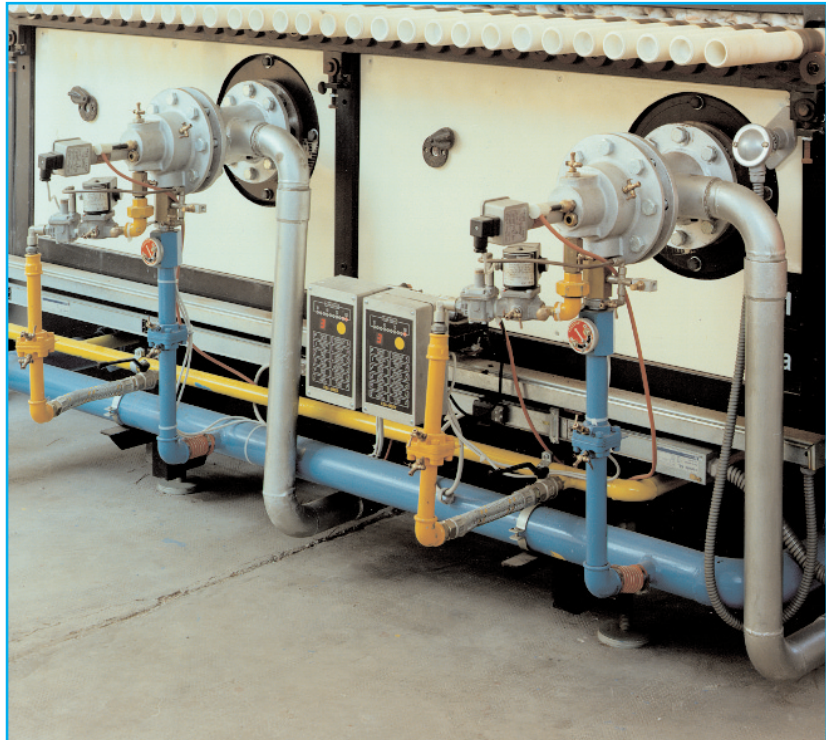
Glass tempering furnace with recuperative, radiant burners, model SER (Poppi Eurotech)
