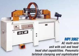
head shot capabilities. Pneumatic tailstock clamping and sophisticated de-mag capabilities have made this machine the automotive crankshaft testing standard for many years. Bed lengths up to 100" and optional 20" coil allow testing of large industrial shafts and components.
