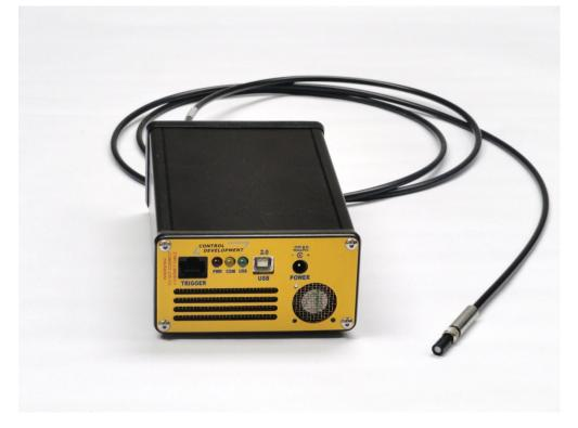
CDI Light meter is the ideal instrument for the measurement of lamps, fluorescents, LEDs, LED chips and flat panel displays. Measure spectral irradiance (w/m<sup>2</sup>/nm), absolute intensity, chromaticity (CIE 1932 2° or CIE 1964 10° observer), L a b color coordinates, correlated color temperature and color rendering indices. Included software also contains peak detection capabilities, derivatives and smoothing functions.
