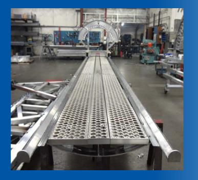
Designed and fabricated out of 6061-T6 aircraft aluminum with custom Aluminum Perf-O-Grip Planking and a 2,722 kg (6,000 kg) net capacity aluminum frame with rails to support trolley
