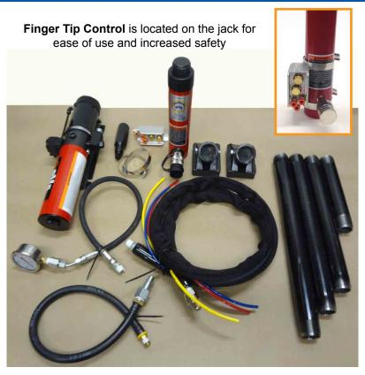
Pneumatically operated hydraulic jack with pressure gauge assures consistency for better quality control.
