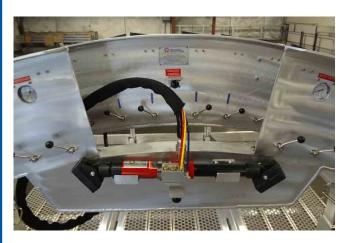
The Long jack is located on cut out section of arch for easy access.
