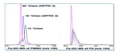
Py-GCMS Chromatogram of PMMA
