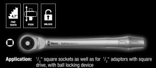
**Design:** Forged, full metal ratchet (chrome-molybdenum) that is extremely robust with a long service life; slim design to enable work in very confined spaces; the dual-ratchet-teeth design means that a 76 fine-toothing division can be achieved from the 38 robust teeth with a return angle of only 4.7°; simple direction change with the undetachable push-through square and very secure socket lock mechanism
