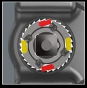
**Double pawl mechanism** A double pawl mechanism and a return angle of only 6° allow you to tighten and loosen screws quickly and accurately even in cramped conditions.
