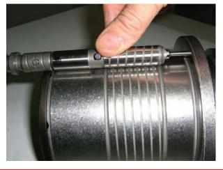
Quickly adjust the length of your punches by using the built-in length guide. Place the tip of the punch against the flange and rotate the punch driver to the guide body edge
