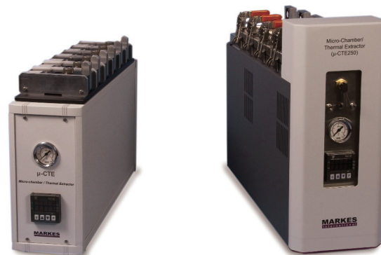
Figure 2. (Left) \mu -CTE with 6 x 44 mL micro-chambers. Max. temp: 120°C. (Right) \mu -CTE with 4 x 114 mL micro-chambers. Max. temp: 250°C
