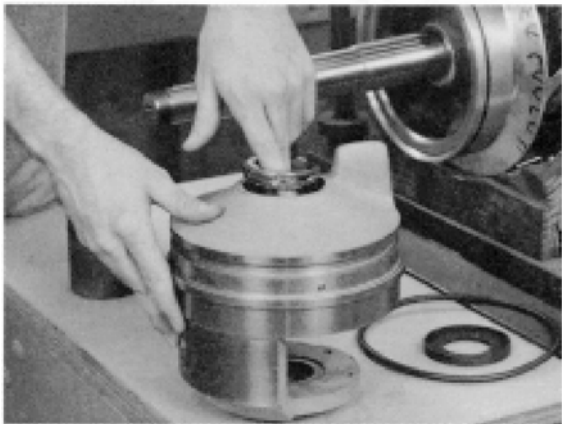
FIGURE 35 – INSTALLING STATIONARY SEAT
