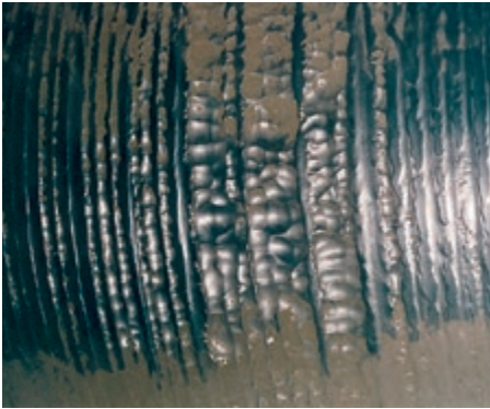
Welded (hard-faced) roll surface after 2,500 hours of service (left) and HEXADUR®-protected surface after surpassing 50,000 hours of service (right)
