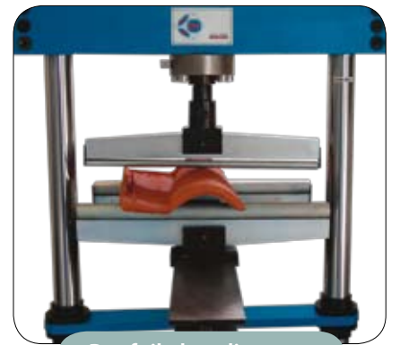
Roof tile bending test
