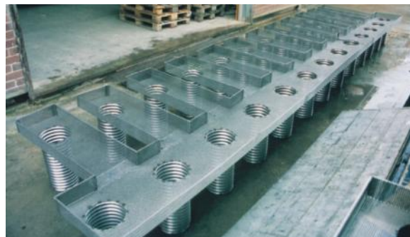
Special casing for machine foundation
