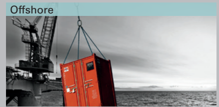
Welded chain slings and master links acc.DNVGL-ST-E271
