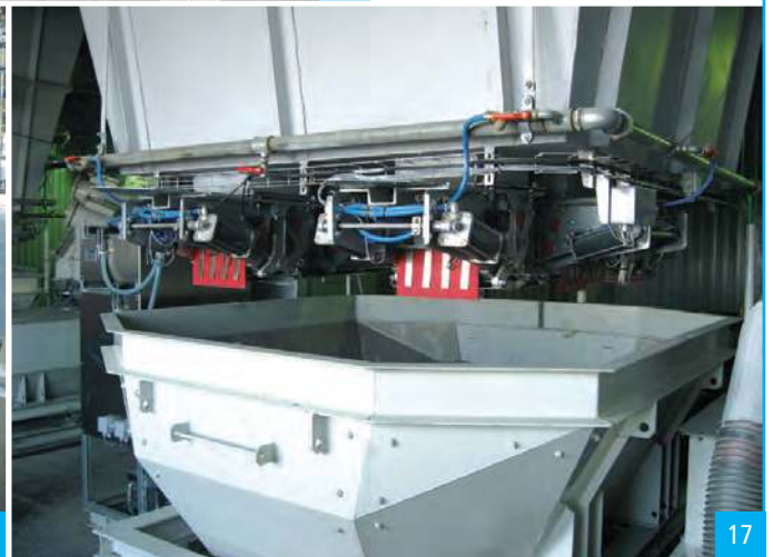
Pict. 14: Segmental dosing gates for aggregates. Pict. 15: Dosing belts for volumetric or gravimetric aggregate dosing. Pict. 16: Aggregate weighing belt with distribution into 2 skip hoist buckets. Pict. 17: Aggregate weighing scale. Pict. 18: Weighing belt for stationary weighing. Pict. 19: Feeding of 2 mixers by means of a two-way distribution gate for aggregate weighing scale Pict. 20, 21: Skip hoists with bottom discharge or tilting buckets
