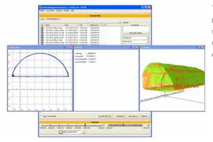
The profile excavated can be shown using the production data of the SLS Roadheader navigation system. The hull calculated in the SLS Roadheader navigation system from all touch points of the excavation tool is used as the basis.
