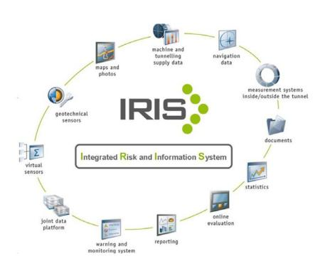
VMT offers with IRIS (Integrated Risk and Information System) a modular and web based multi user system whose acquisition, analyzing and evaluation functions are specifically developed for mechanical tunnelling.
