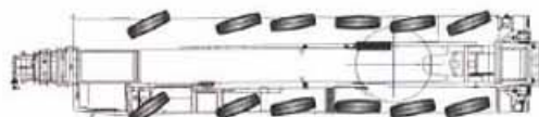
前后桥同向转向：蟹行行走 Front and rear axles synchronous steering: Crabbing walk
