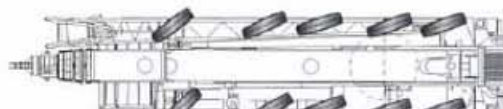
前后桥同向转向：蟹行行走 Front and rear axles synchronous steering: Crabbing walk
