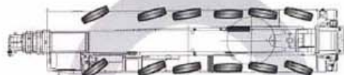
前后桥反向转向：小半径转弯 Front and rear axles reverse steering: Small radius turning 24m
