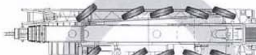
前后桥反向转向：小半径转弯 Front and rear axles reverse steering: Small radius turning 18m
