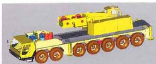
55吨自重行驶状态 Crane travel with 55t dead weight
