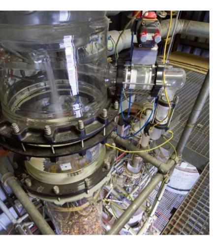
In the amine recycling plant this process takes place in the reactor. The amine released is cleaned by column rectification and transformed into a usable condition with a high degree of purity. The resultant amine is then filled into containers approved for this purpose and returned to use through the foundry supply industry.
