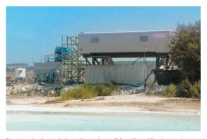
Even treating large sludge volumes is possible with mobile plants – in part we can produce up to 300 t filter cakes per shift
