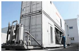
The nitrogen covering means no explosive zone can arise within the gas-tight decanter from FILTRATEC. The three phases of oil, water and solid result in only one step
