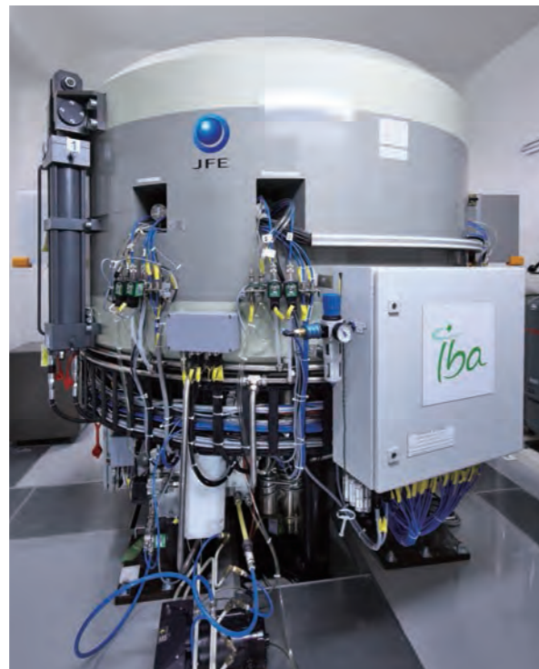
◇ Cyclotron / Produces radioactive substances used in PET (Positron Emission Tomography) examinations.
