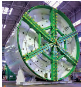
◇ Shield machine for tunnel construction
