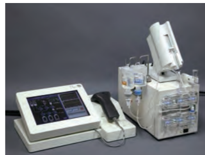
◇ PET test drug synthesis system / Produces radioactive drugs.
