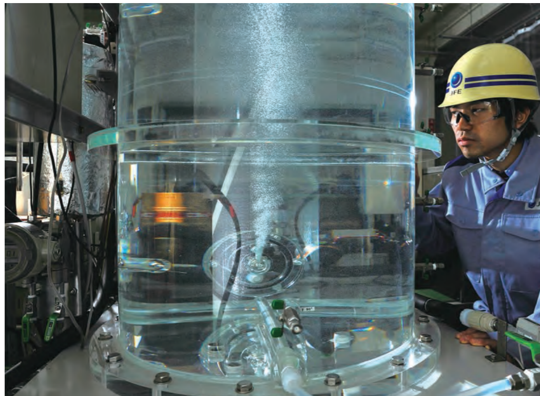
◇ Fluid test / Visualizes the condition of fluids in containers provides information for use in the design of internal structures, etc.
