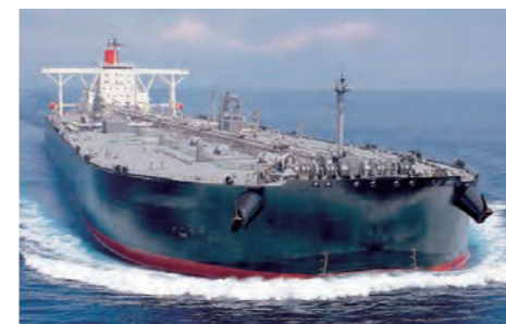
◇ Oil tanker equipped with JFE’s “Ballast Ace®” ballast water management system
