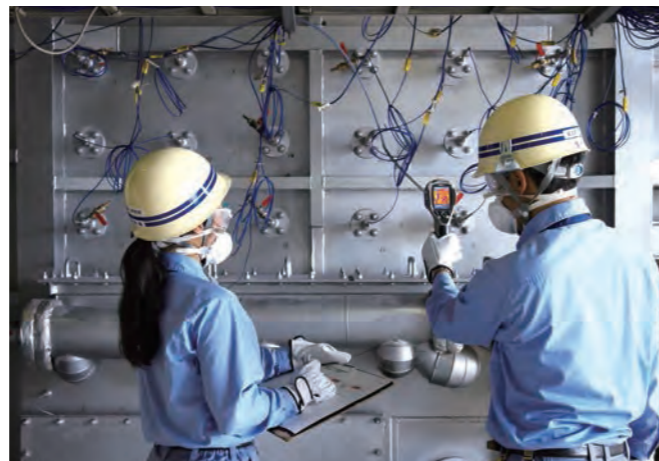
◇ Waste combustion test / Conducts various types of combustion tests for achieving even higher performance in waste plants.
