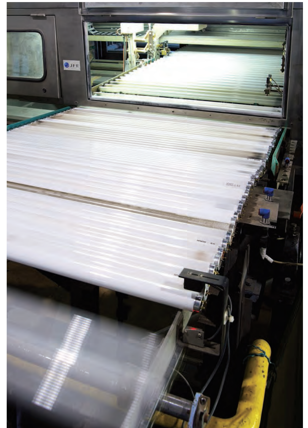
◇ Fluorescent Light Tubes Recycling Factory (Kanagawa Pref.) / Fluorescent powder and mercury are removed, and the glass is recycled.
