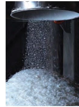
◇ Flakes recycled from PET bottles. These flakes will become the raw material for textiles products, etc.
